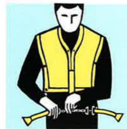
STEP 2 Fasten the rings on the waist strap ends to the snaps at bottom front of the vest; then grasp the pull tabs on the waist strap ends and pull snug around your waist.
