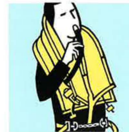
STEP 4 If the vest becomes too soft later, blow into the two rubber tubes.
