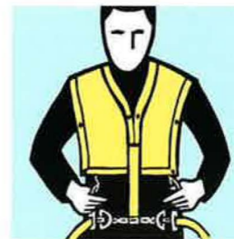
STEP 3 After you leave the plane, inflate vest by pulling sharply on the two cords at bottom.
